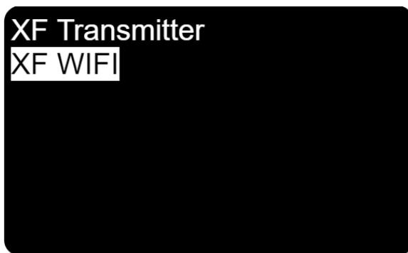
Connect your CROSSFIRE/ TRACER to a hotspot via the built-in WiFi module. You can provide access point information from your nearest wifi hotspot, or create a temporary one on your phone. Connect your PC to the same network. **OR** connect your PC/ mobile phone straight to the CROSSFIRE/ TRACER access point.
